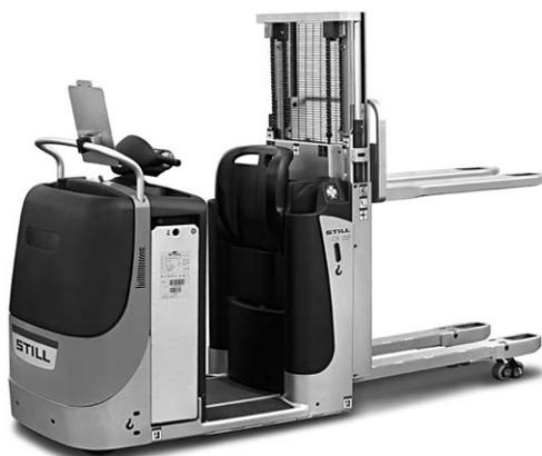
Double-deck forklift truck for high storage density
