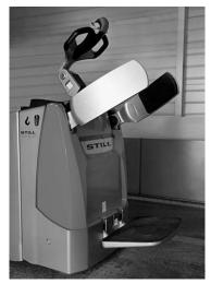
Adjustable height side guards and ergonomic tiller optimally designed for driving,.
