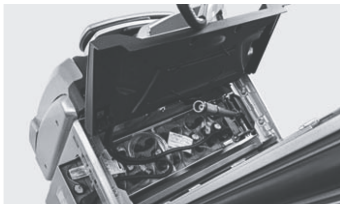
Fast and safe: innovative battery plug lock enables fast battery replacement, without the risk of jamming
