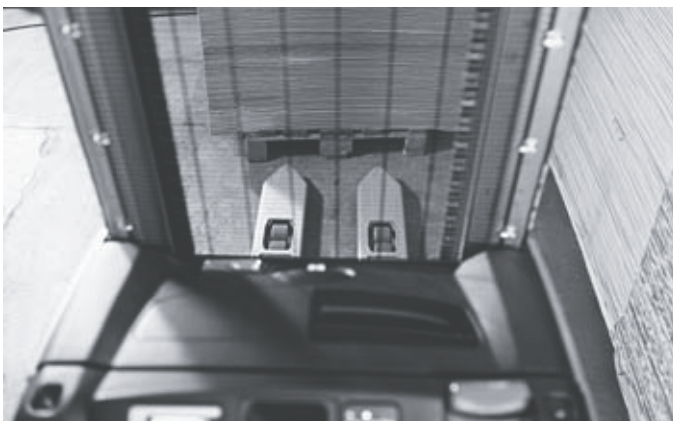
STILL free view mast always ensures the best view of the tips of the forks
